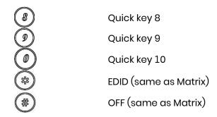
For example: to connect output port 1 to input port 4, press the quick key 1 (OUTPUT 1) and then press the quick key 4 (INPUT 4).
