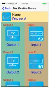
Yellow block shows matrix name and icon Green block shows name and icon of output devices Brown block shows name and icon of input devices
